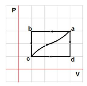
3. An ideal gas can be taken from state a to state c in three different paths: a→b→c, a→d→c, and curved path a→c. The pressure of the ideal gas at point a is three times the pressure at point d. Use the following information to answer all questions:
