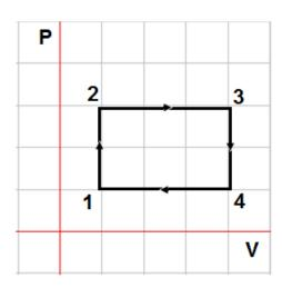
31. The state of an ideal gas is changed in a closed path  $1\rightarrow2\rightarrow3\rightarrow4\rightarrow1$ . Which of the following is true about work done on the gas?
